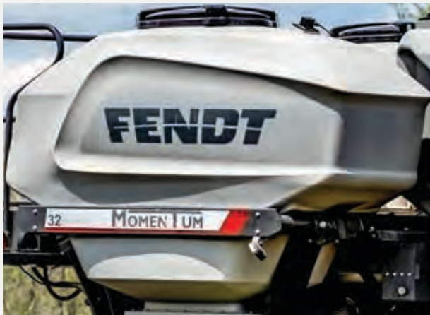
Twin 65-bushel seed tanks for a total of 130-bushel capacity and is easily accessed with a wide platform.
